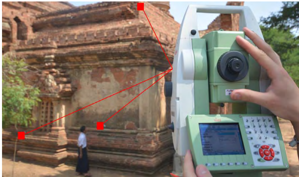
Figure 10 Surveying the targets on the temple employing a Leica Total Station TS11. Source: Author.
