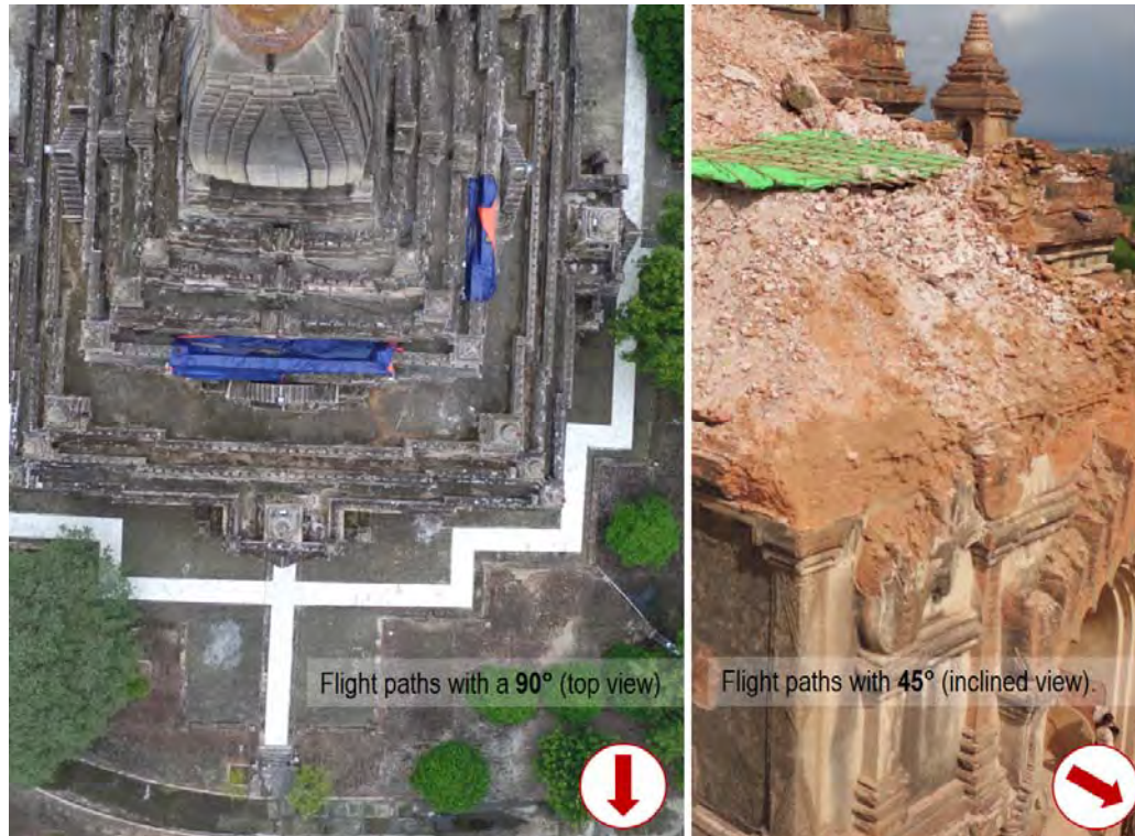
Figure 23 Image showing different drones' camera orientations to capture different information of Bagan temples. Source: Author.
