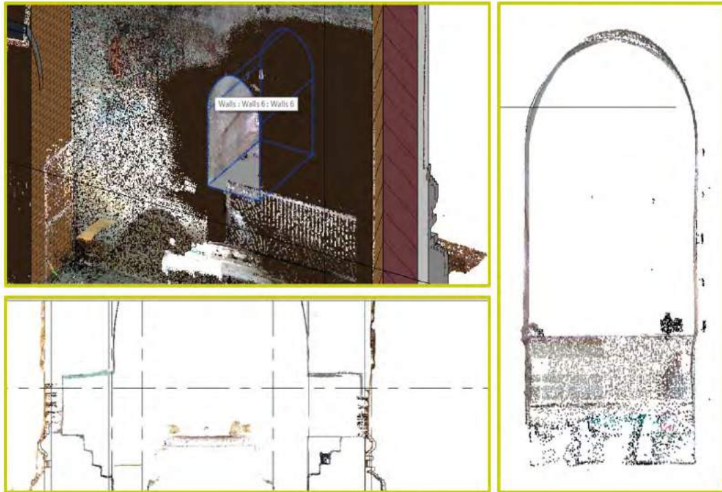
Figure 16 Image illustrating the voids behind the windows and the modelled window void. Software employed Autodesk Revit2016. Image source: Author.
