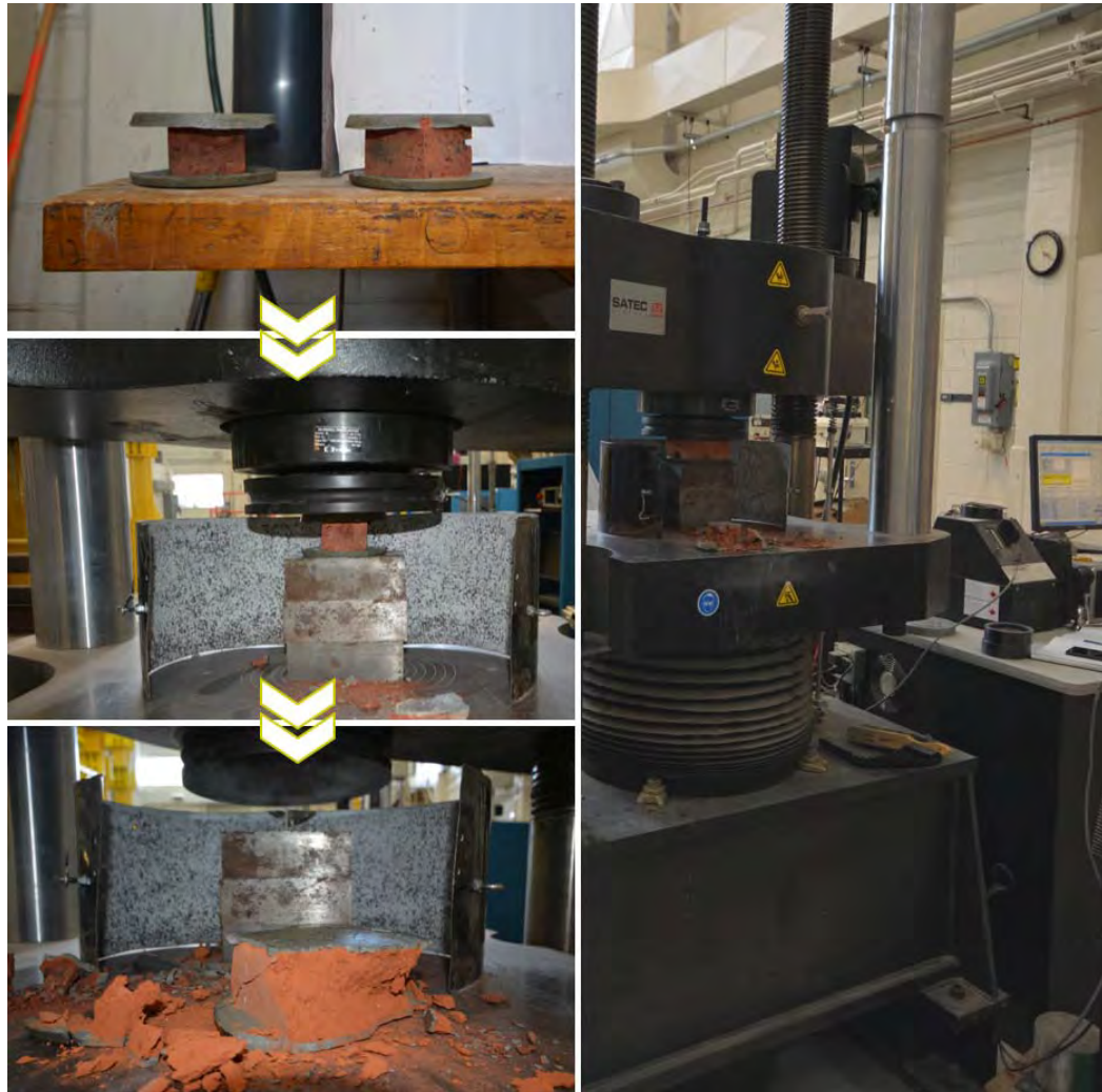
Figure 44 Images illustrating the three main steps followed in the compressive strength test carried out on the samples of the ancient and new bricks. Image source: Author.
