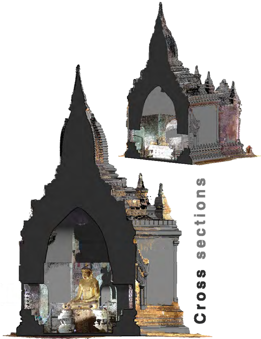
Figure 38 Screenshot of the sectioned Revit model of the temple. Software employed Autodesk Revit2016. Image source: Author.
