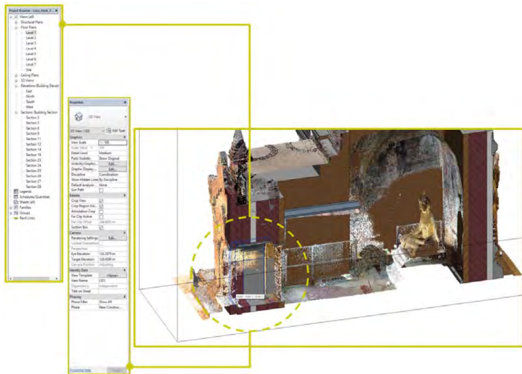
Figure 15 Image illustrating the entrance voids in section view. Software employed Autodesk Revit2016. Image source: Author.
