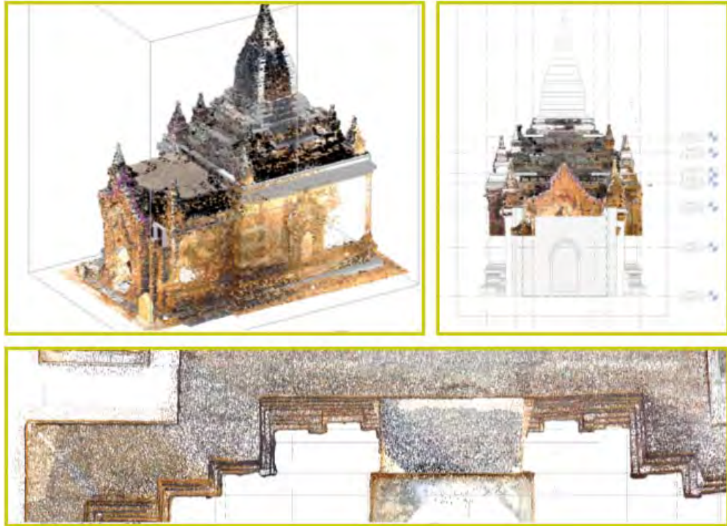
Figure 5 Image illustrating the use of the levels as reference to model the temple from the pointcloud. Software employed Autodesk Revit2016. Source: Author.
