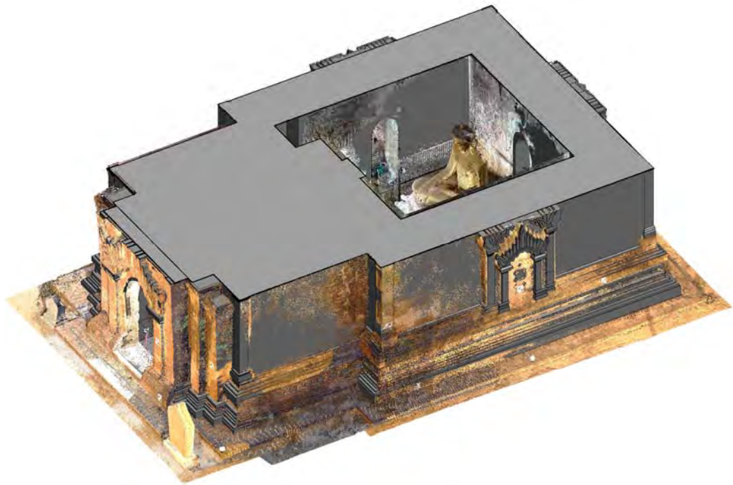
Figure 37 Screenshot of the sectioned Revit model of the temple. Software employed Autodesk Revit2016. Image source: Author.
