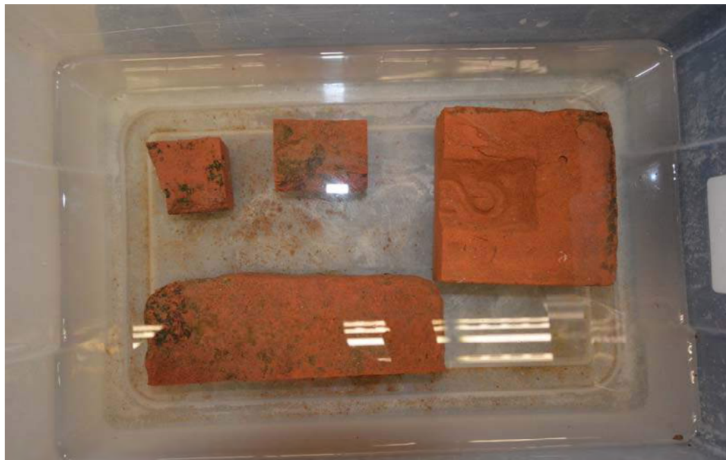
Figure 45 Image illustrating the cold water absorption test in progress. Image source: Author.
