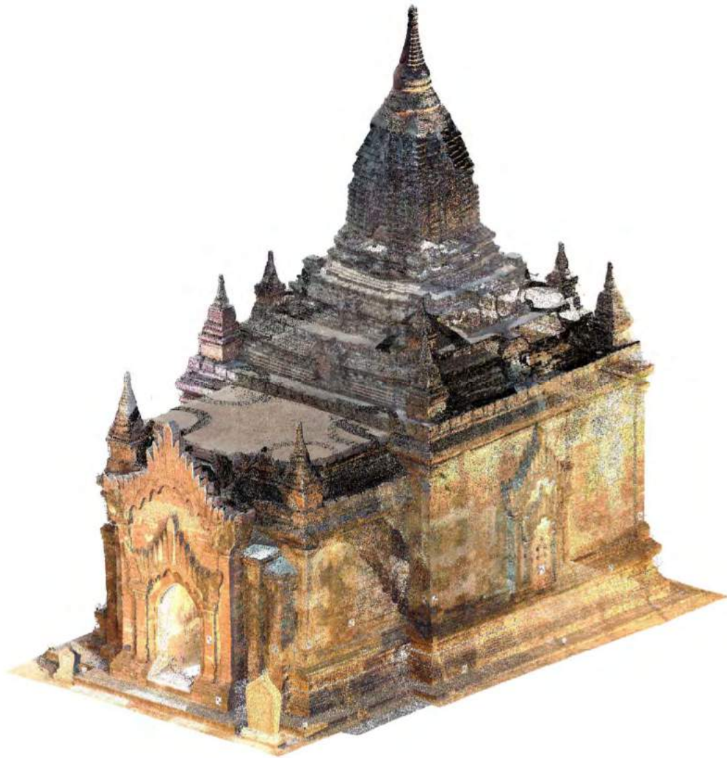
Figure 38 Screenshot of the ReCap model showing an exterior axonometric view of the Lokateik-pan temple pointcloud. It has been generated combining photogrammetric and laser scanning data. Source: Author.
