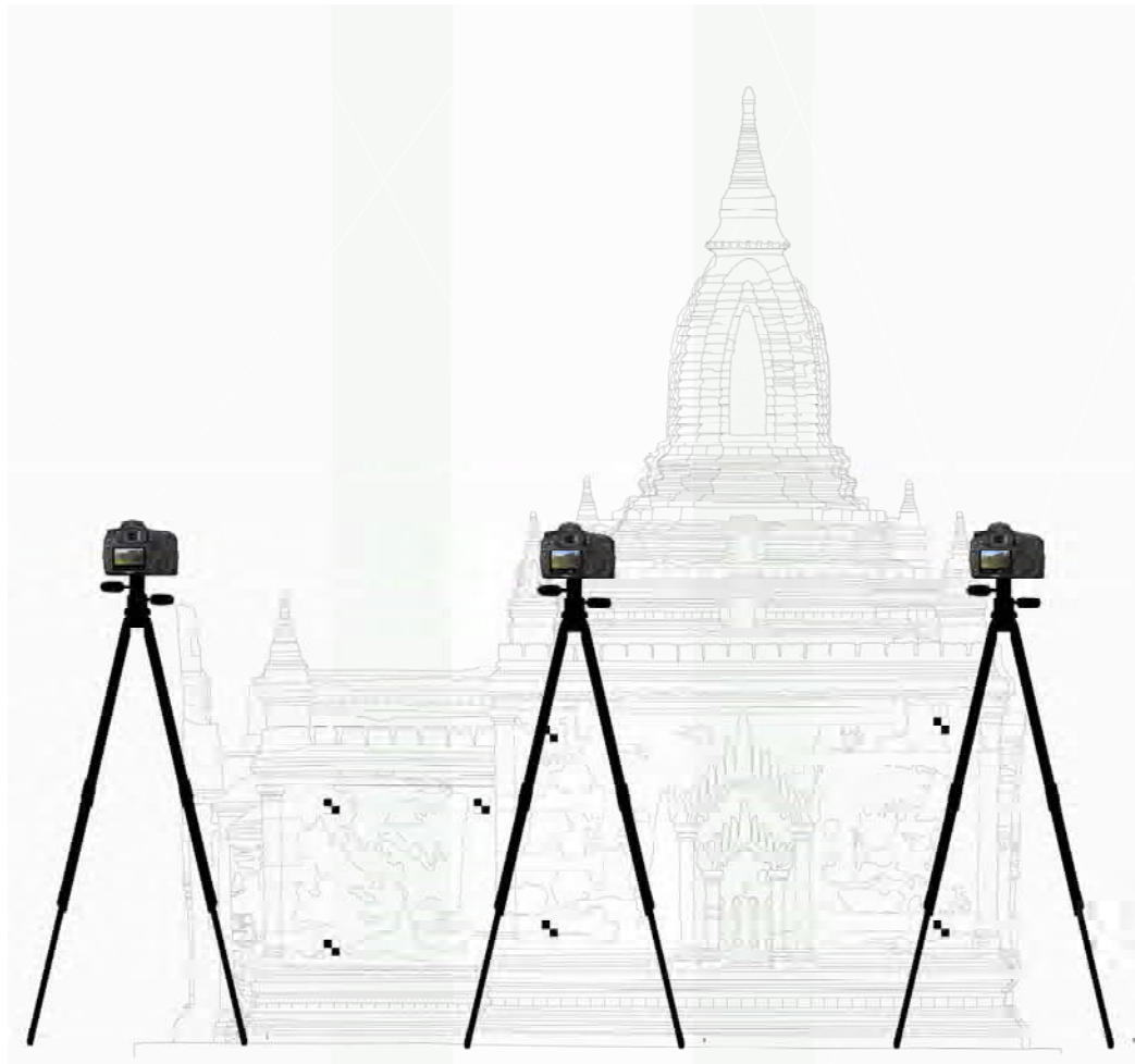
Figure 15 Image illustrating the use of the tripod to take photos at different heights and from different distances from the Loka-hteik-pan temple to gain information of the different parts of the building. The tripod has been useful to avoid blurry photos. Image source: Author.
